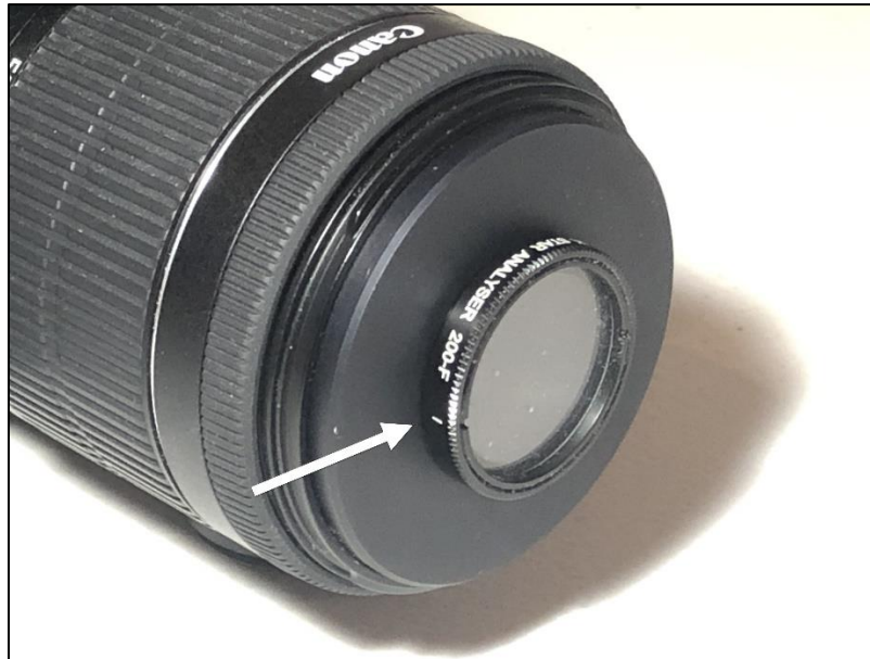
Grating with alignment mark properly positioned
