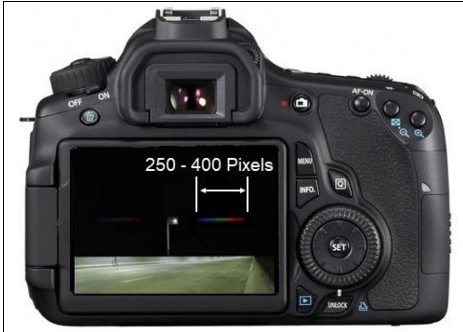
Above: Street light with grating properly rotated and good zoom
