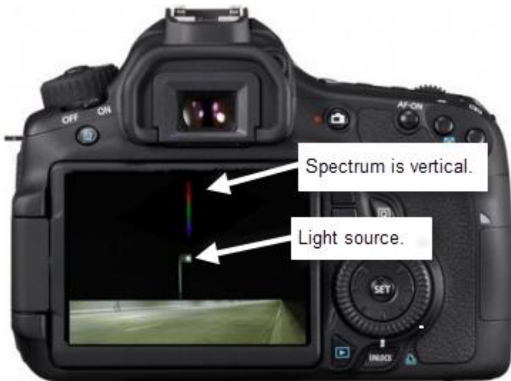
Figure 2. When the grating is mounted in the proper rotation, a spectrum appears vertically above a compact light source.
